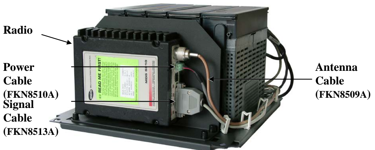
Figure 21-86 MDS Radio Modem Installed on ACE3600 Chassis – Cable Connections
