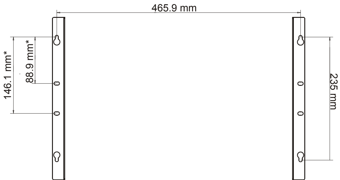
Figure 2-10 8 I/O Frame (19") Metal Back Installation Dimensions
