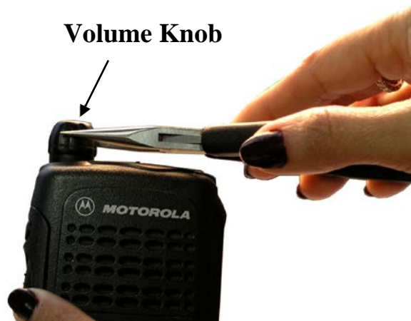
Figure 21-38 Removing the Volume Knob
