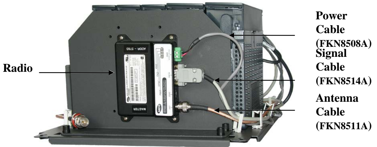
Figure 21-75 TransNET 900 Radio Modem Installed on ACE3600 Chassis – Cable Connections
