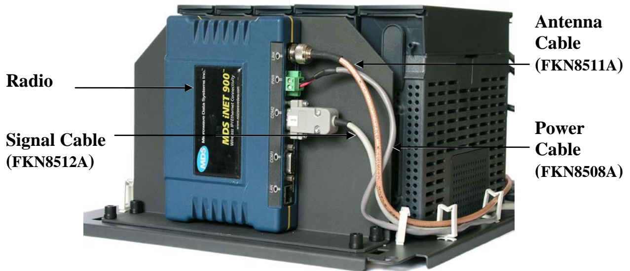
Figure 21-80 iNET 900 Radio Modem Installed on ACE3600 Chassis – Cable Connections
