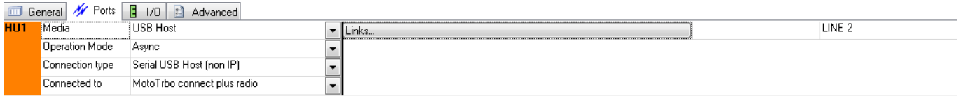
Figure 21-66 MotoTrbo Connect Plus Mode – RTU LINE 2 Configuration
