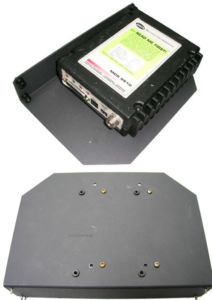
Figure 21-84 MDS Radio Mounted on Metal Bracket - Front and Rear View
