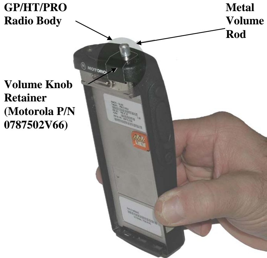
Figure 21-40 Attach Retainer to Radio
